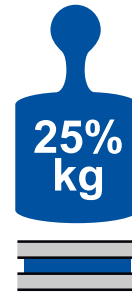
Horizontally mounted = 25% quoted load rating
