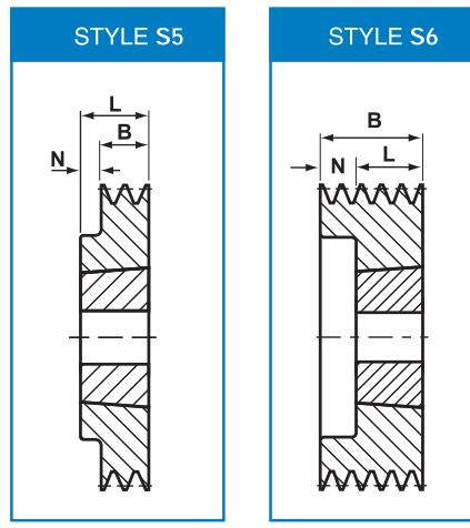
Pulley Configuration: S = Solid, P = Plate , A = Arm.
