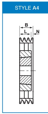
Pulley Configuration: S = Solid, P = Plate, A = Arm.
